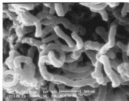
Figure 1. SEM image of the carbon nanotubes grown by means of CCVD using \text{BaCl}_2/\text{CaCl}_2 catalyst support.
